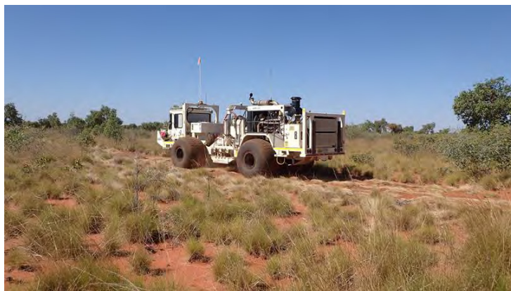
Figure 11: Example of a vibroseis truck used during seismic acquisition
