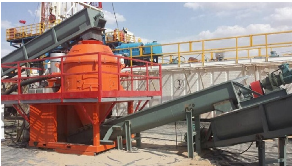
Figure 19: Example of a cuttings dryer used to recover synthetic based drilling fluids
