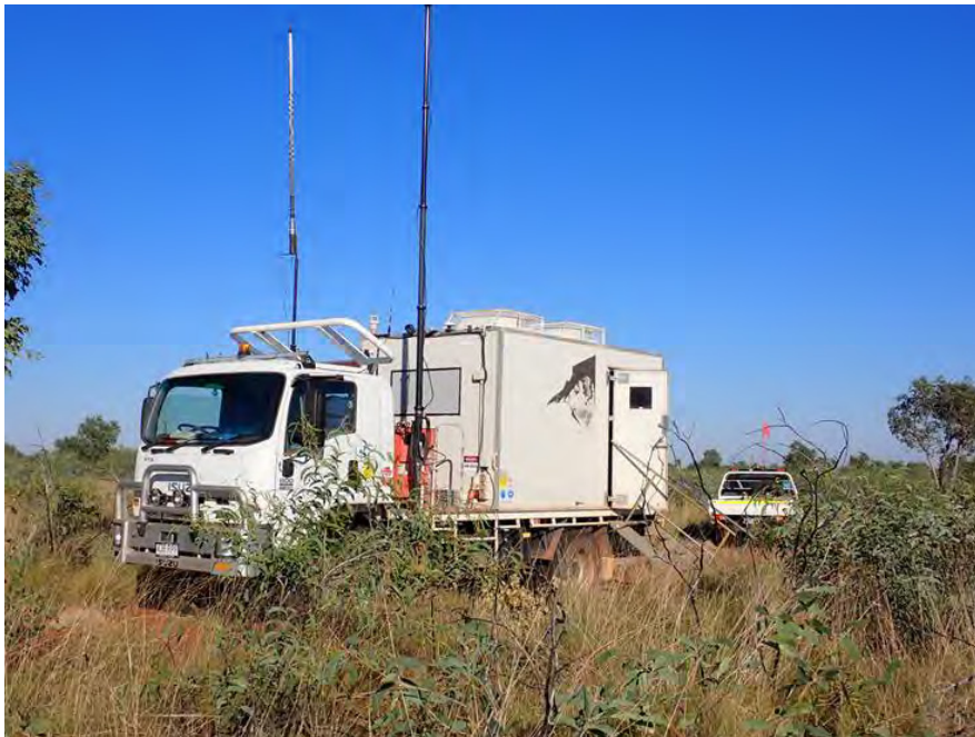
Figure 12: Data recording van used during seismic acquisition
