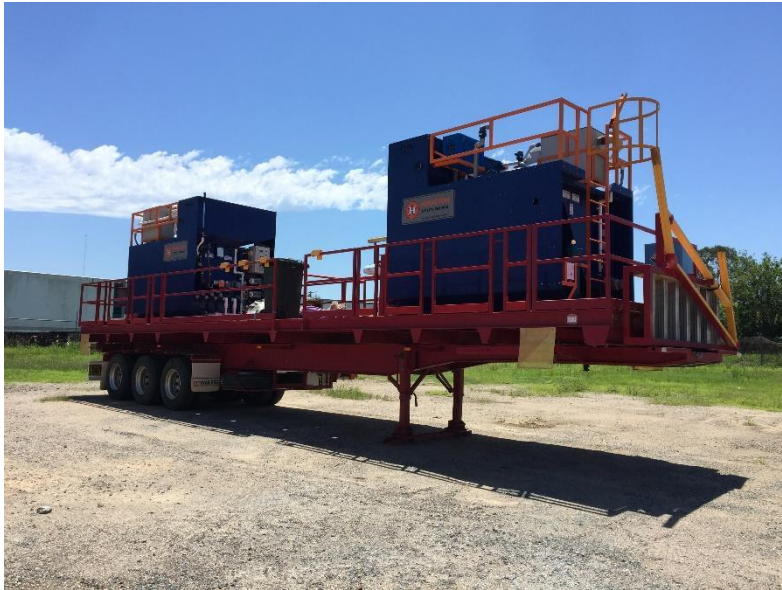
Figure 4-7. Example of wastewater treatment used at mobile camps
