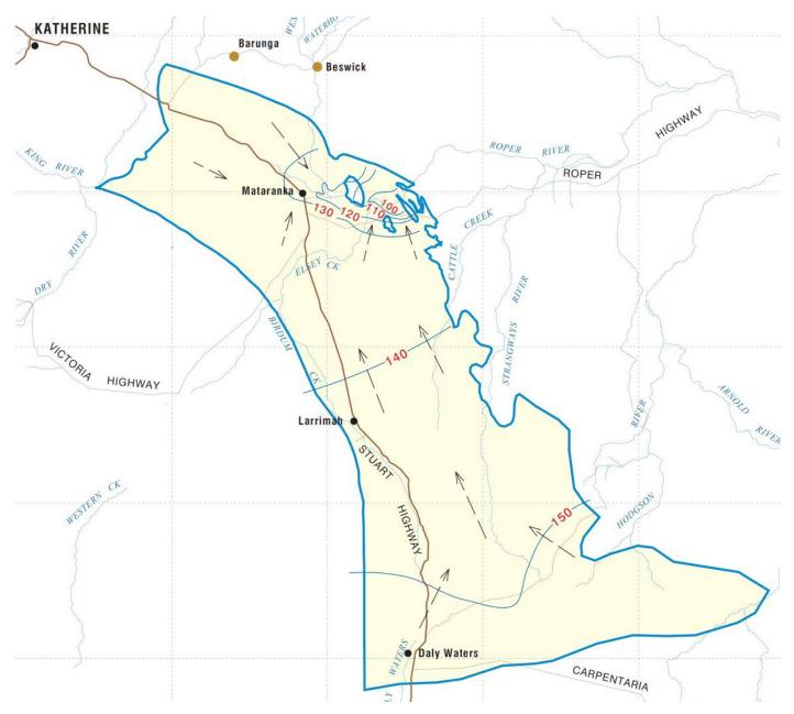
Figure 5 Groundwater flow directions in the Tindall Limestone Aquifer, Mataranka – Daly Waters (figure from Bruwer & Tickell, 2015). The groundwater flow directions are indicated by arrows. Numbered lines show the groundwater levels (in meters AHD) in the aquifer. The groundwater flows from areas where levels are higher, towards areas where levels are lower.
