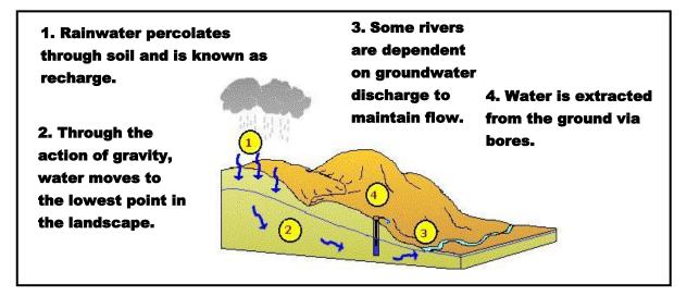
Figure 3 Conceptual Groundwater Diagram
