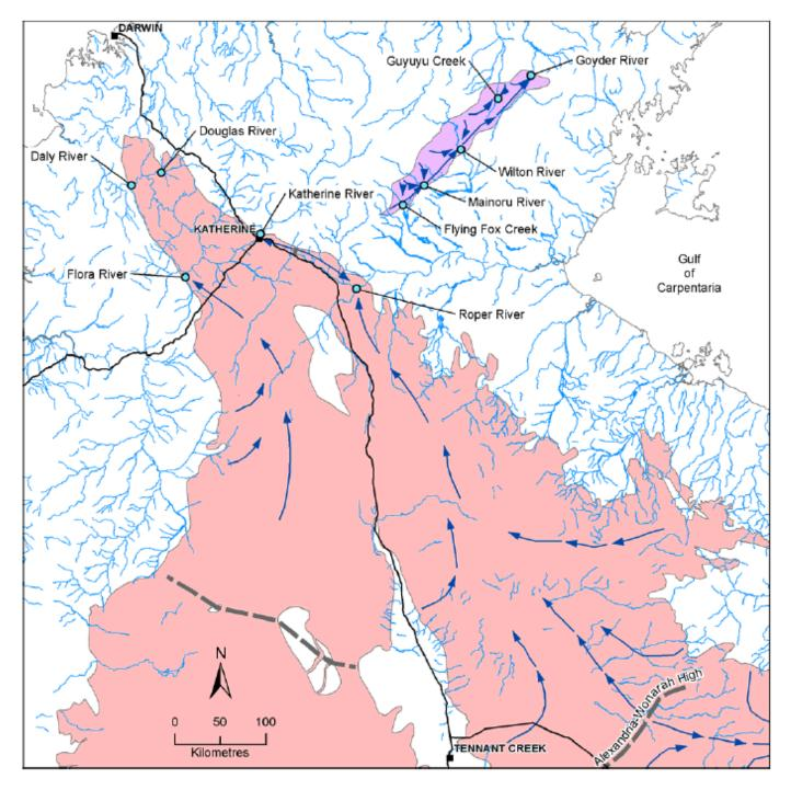
Figure 8 Regional groundwater flow in the Cambrian Limestone aquifer (Tindall Limestone Aquifer, Gum Ridge Formation and Montejinni Limestone) and the Dook Creek Formation (Figure from Knapton, 2009 Part A). Arrows indicate the direction of groundwater flow. Groundwater discharges from these aquifers contribute to flows in the Roper River.
