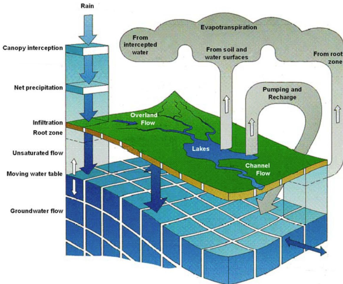
Figure 28 Conceptualisation of Mike SHE modelling components. In this case the groundwater flow was modelled using FEFLOW.
