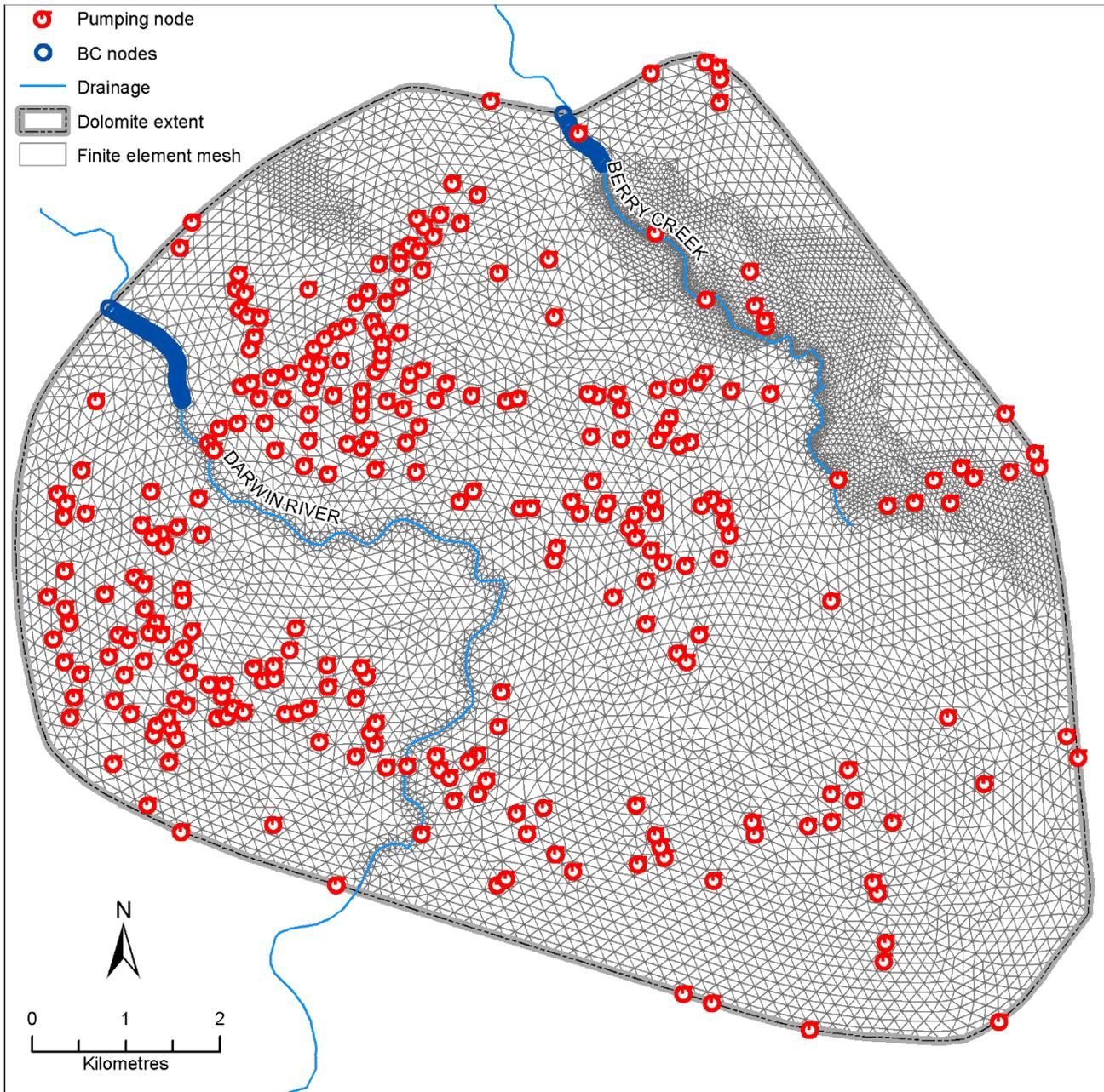
Figure 23 Location of pumping nodes applied to slice 3 of the FE model.
