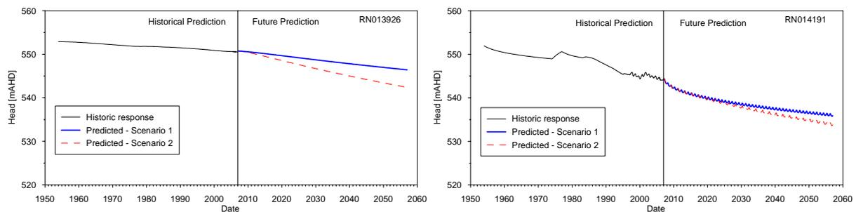
Figure 8 Predicted water levels in response to pumping at TGA a) RN13926 and b) RN14191.
