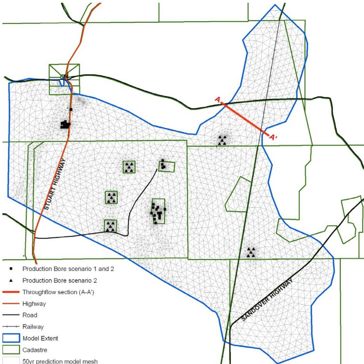
Figure 6 Geometry of finite element mesh with locations of the borefields for future horticultural regions. A-A' indicates the location of the section used to determine variations with throughflow.
