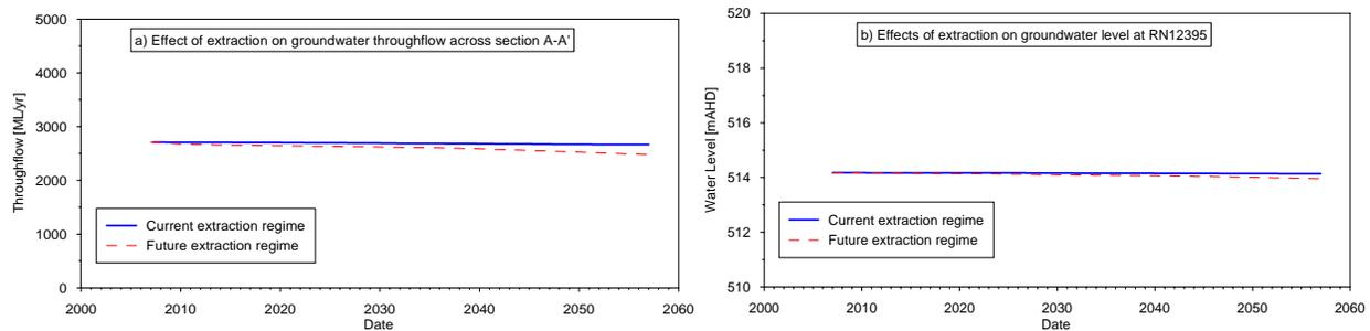
Figure 9 predicted effects of extraction scenarios on a) throughflow to the north and b) water levels at RN12395.
