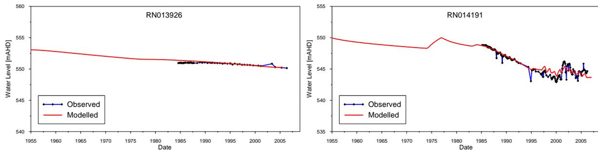
**Figure 5** Comparison of the predicted and observed groundwater levels in the vicinity of the Table Grape Growers of Australia borefield.
