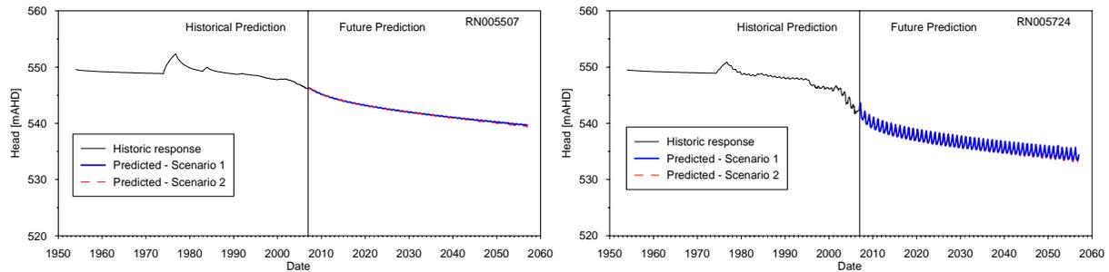
Figure 7 Predicted water level in response to pumping at TTF a) RN5507 and b) RN5724
