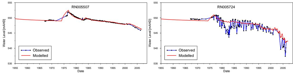
**Figure 4** Comparison of the predicted and observed groundwater levels in the vicinity of the Ti Tree Farms borefield.
