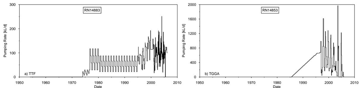
**Figure 3** Examples of historic pumping schedules for a) Ti Tree Farms and b) Table Grape Growers of Australia
