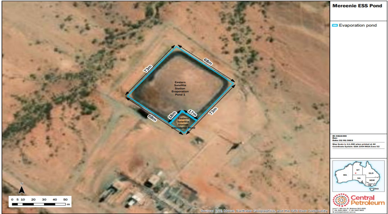
Figure 3-9: ESS Wastewater solar evaporation ponds
