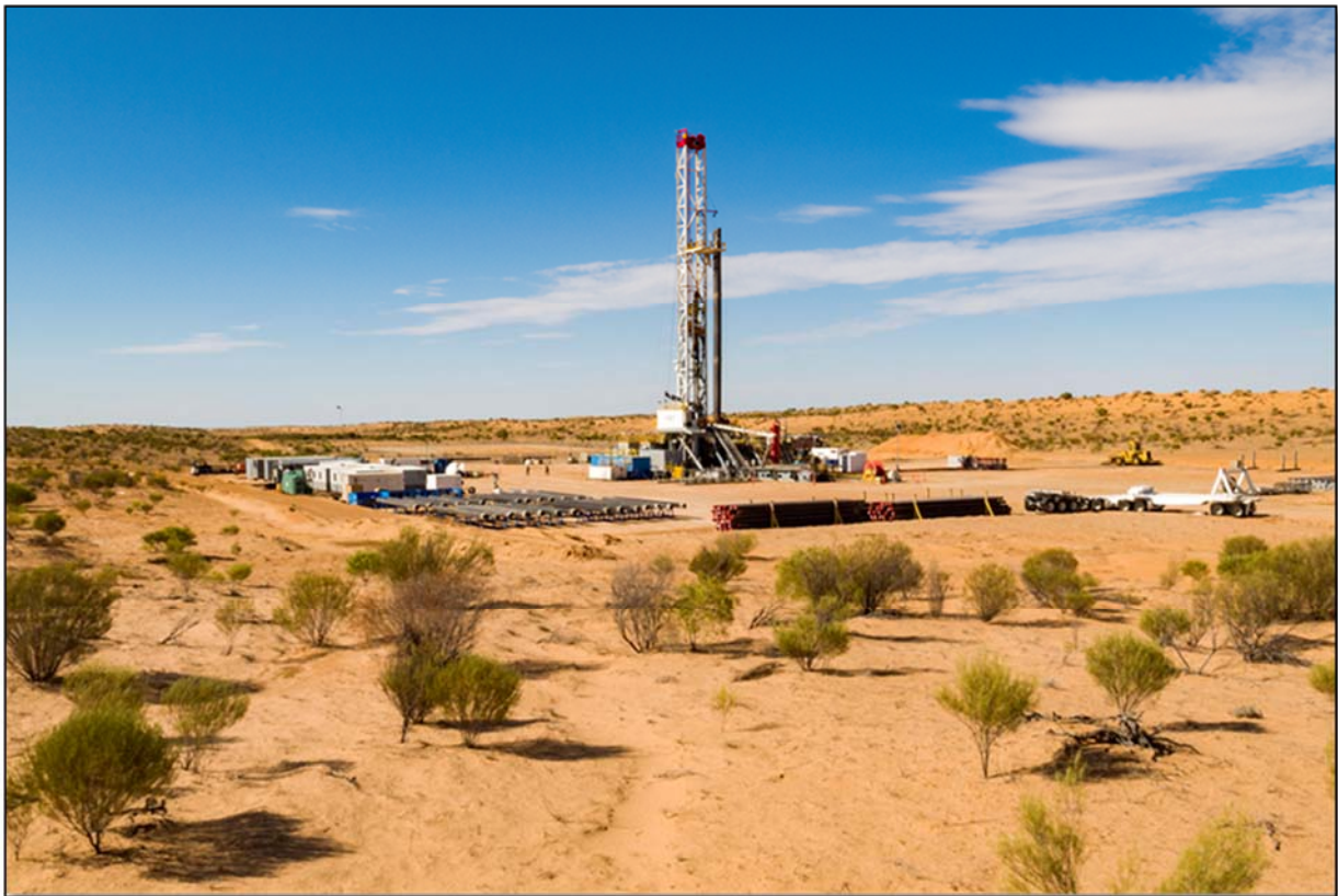
Figure 3-4: 1500HP (horse-power) triple drilling rig
