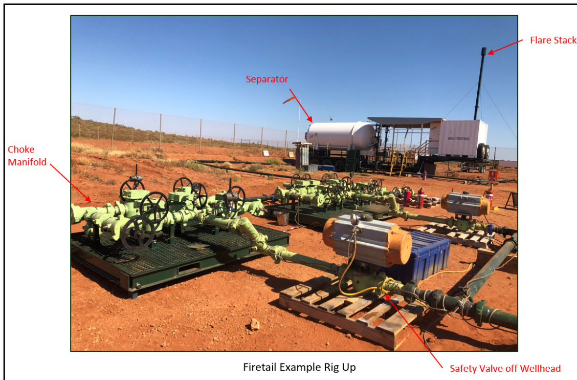
Figure 3-27 Example Well testing Flare Set Up.
