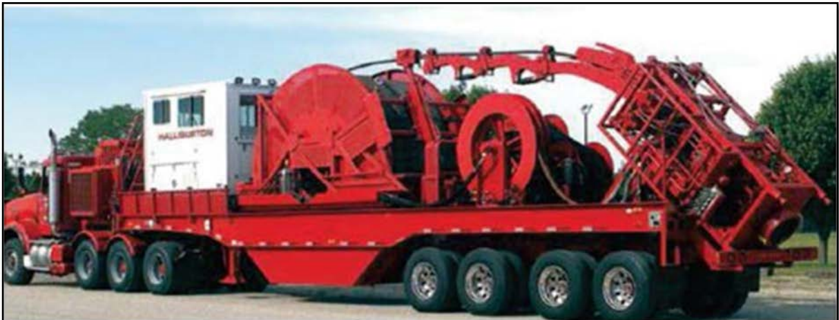
Figure 3-28 Coiled tubing unit. (Halliburton 2012)
