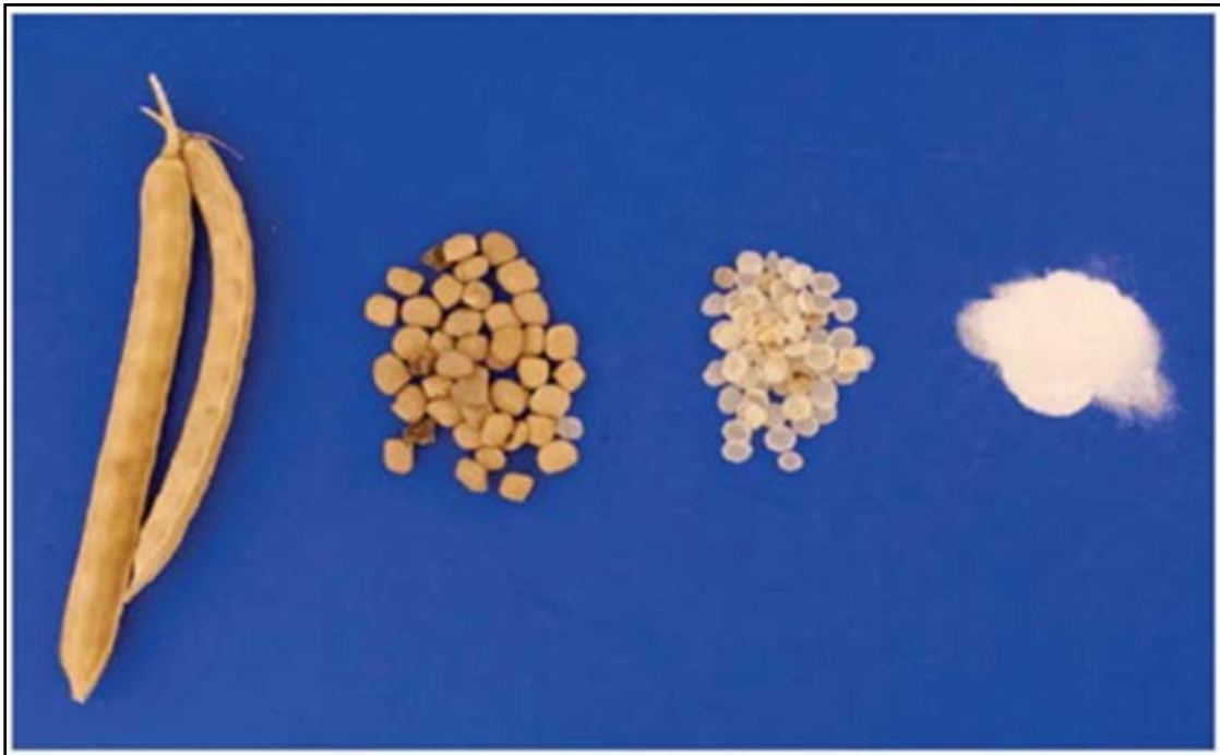
Figure 3-16 Guar gum in its native form, seed form, splits and powder. (Economides and Martin, 2007).
