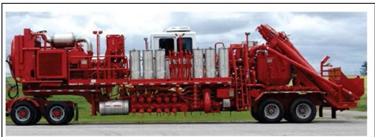
Figure 3-23 Blender unit. (Halliburton 2012)
