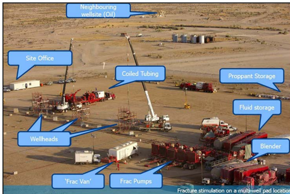
Figure 3-13 Fracture Stimulation equipment in a 3-well location (pad) in the Cooper Basin
