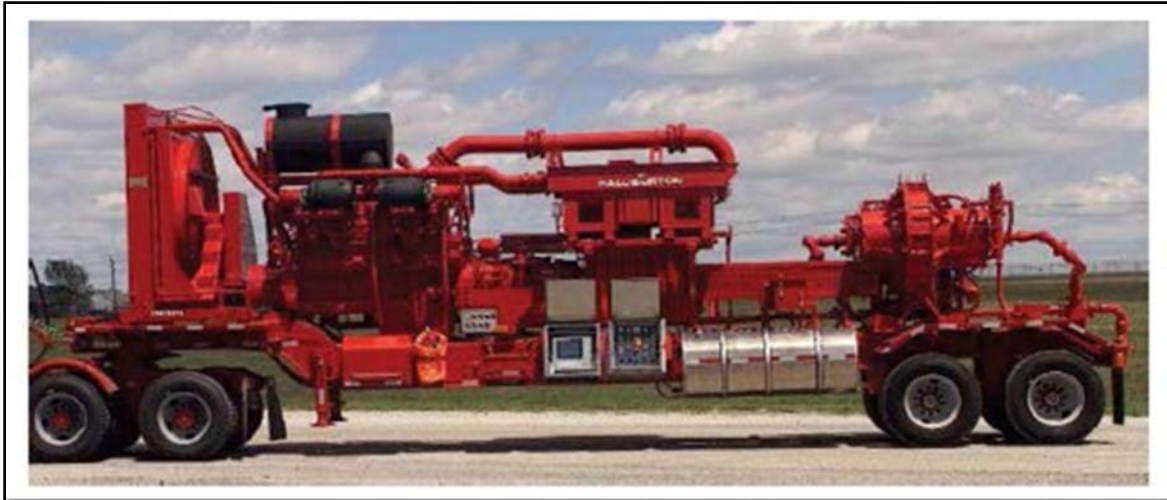
Figure 3-24 High pressure pump. (Halliburton 2012)
