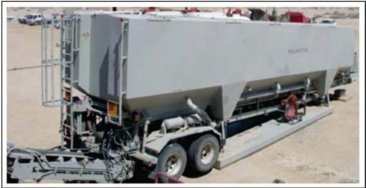
Figure 3-22 Sand trailer unit. (Halliburton 2012)
