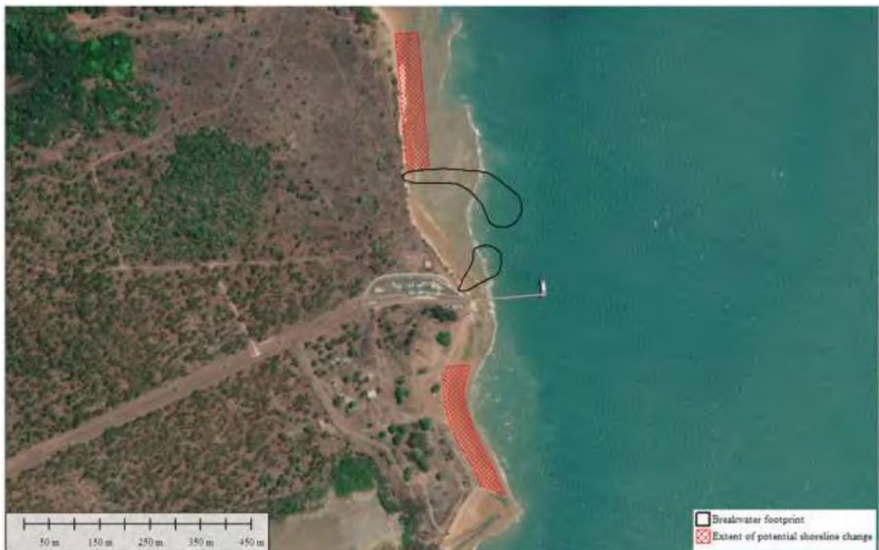
Figure 2 Extent of predicted shoreline change; sediment accretion to the north and erosion to the south
